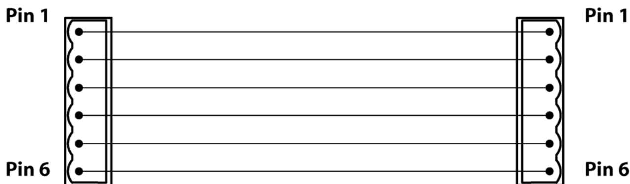
Figure 29: TB10 Jumper Cable Wiring
