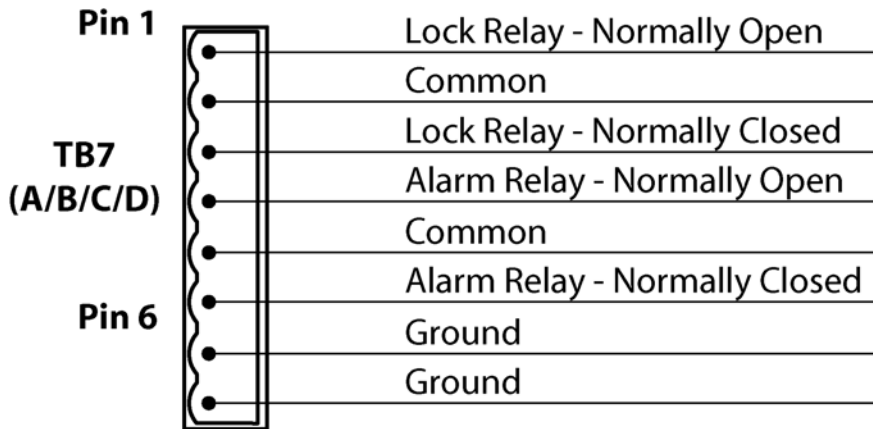
Figure 14: B-Door Lock Relay and Alarm Relay Connections
